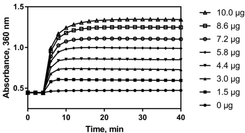
**Figure 3.** Increase in absorbance at 360 nm on incubation of 0-10 µg of phosphate per test
